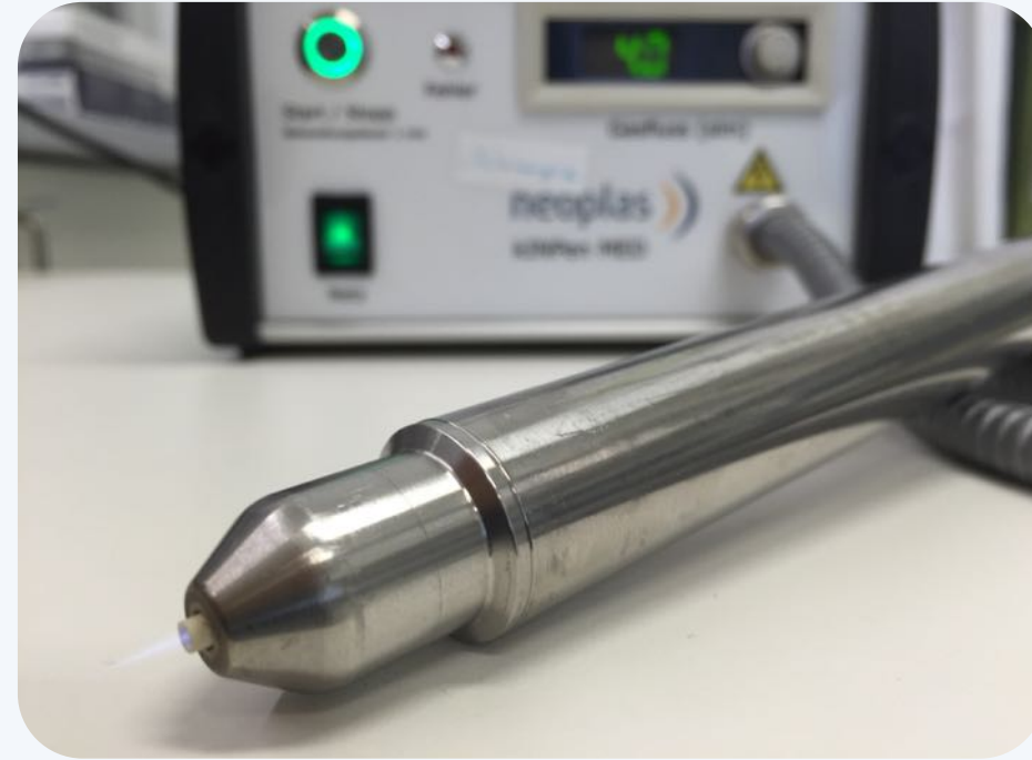
Fig. 1: The kINPen med served as a plasma source. It generates an atmospheric pressure non thermal jet-plasma and was fed with Argon at three standard-litre per minute.
